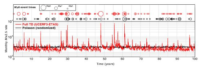
UCERF3-ETAS (red) simulates 100-yr statewide M≥6 events and monthly M≥2.5 rates, showing aftershock decay and clustering, unlike the time-independent Poisson model (black) which randomizes event times, thereby removing spatiotemporal clustering. From Field et al. (2012).
