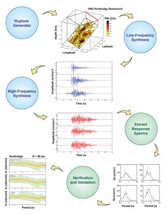
A Broadband Platform workflow showing a simulation method consisting of a rupture generator, low- and high-frequency waveform synthesis, and two stages of post-processing. Modified from Maechling et al. (2015).
