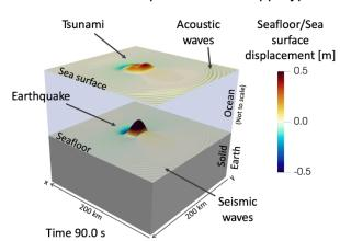
The SeisSol earthquake-tsunami App type allows users to model earthquake-tsunami interaction. Illustrated is a very simple 3D fully coupled simulation output resembling the recent CRESCENT and SCEC/USGS earthquake-tsunami benchmark setup TTPV1, showing a vertically exaggerated view of how the seafloor is permanently displaced due to spontaneous earthquake dynamic rupture, and how acoustic waves and the tsunami propagate at the sea surface.
